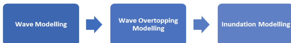
Figure 2-2: Modelling components of the wave overtopping assessment.
